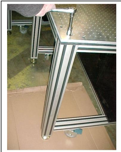
Precise leveling of Robotic Tables is crucial for repeatable robot performance. Top Leveling adjustments make it simple.
