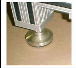
Standard Robotic Tables are equipped with 3" leveling feet. These feet are ball jointed to accommodate for uneven floors.
